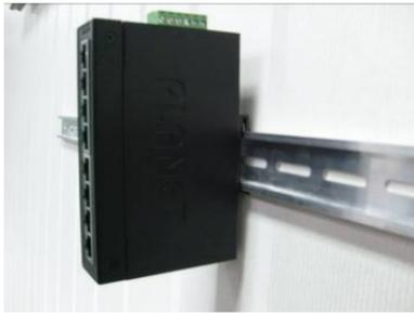
**Step 3:** Check the DIN-Rail is tightly on the track.
