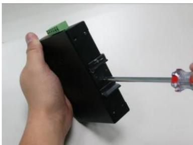
**Step 1:** screw the DIN-Rail on the Industrial 802.3at PoE Media Converter
