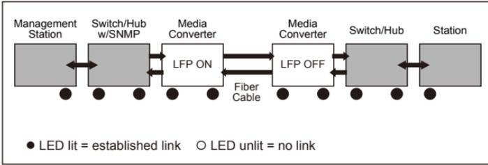
If one of the optical conductors is bad (as shown in the diagram box below), the converter with LLR enabled will return a no-link condition to its link partner. With LLCF also default enabled, the no-link condition is carried forward to the switch/hub where a trap is generated to the management station, and the administrator can then determine the source of the loss.
