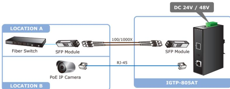
**Figure 2-5:** IGTP- 805AT Stand-alone Installation
