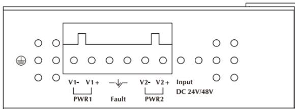
Figure 2-3: Industrial 802.3at PoE Media Converter upper Panel.
