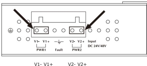
2. Tighten the wire-clamp screws for preventing the wires from loosening.
