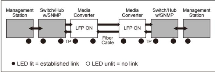
If the connection breaks, IGTP-80xT that link loss forward to the switch/hub which generates a trap to the management station. The administrator can then determine the source of the issue.
