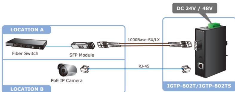
**Figure 2-4:** IGTP- 802T / IGTP-802TS Stand-alone Installation
